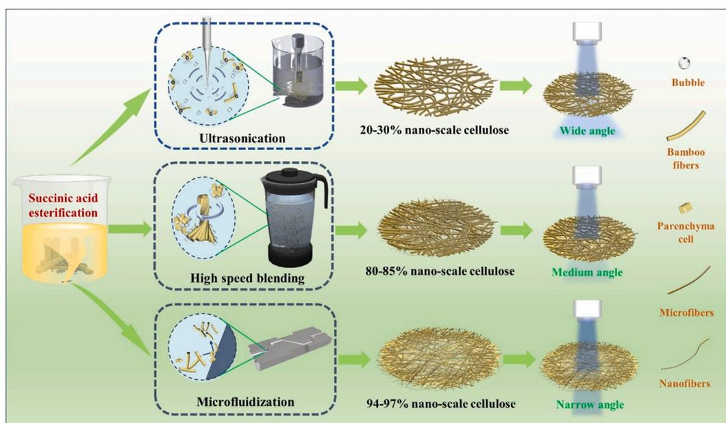
Fig. 7. Mechanism of various mechanical defibrillation and their effects on the optical properties of MNC films.
