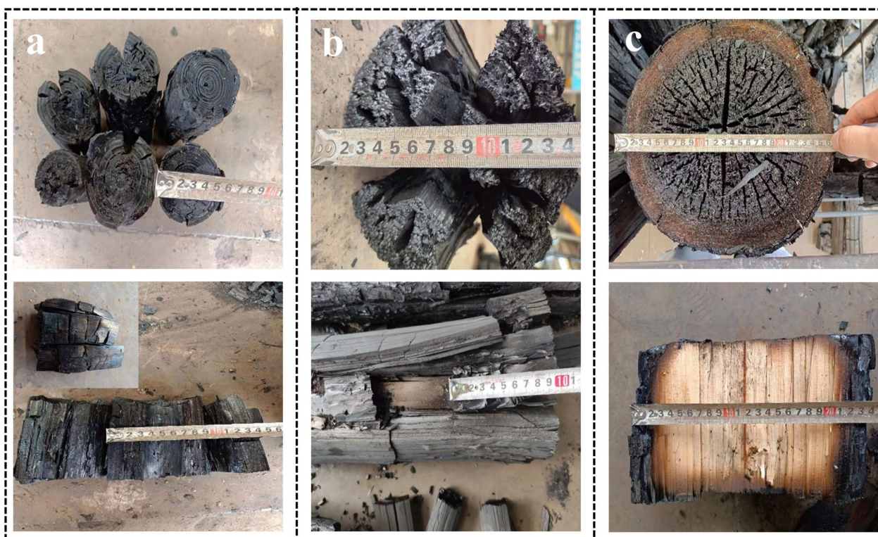
Fig. 7 Appearance of IPW with different diameters after carbonization
